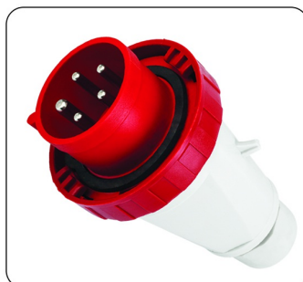
Plug 3P+N+E-16A-6h/415V~ IP66 Code:710
