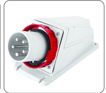
Appliance Inlet 3P+N+E-63A-6h/415V~ IP66 Code:985
