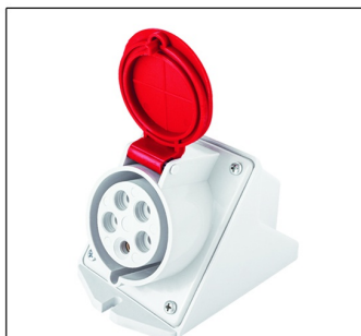
Socket 3P+N+E-32A-6h/415V~ IP44 Code:425
