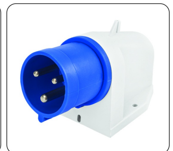
Appliance Inlet 2P+E-32A-6h/250V~ IP44 Code:615
