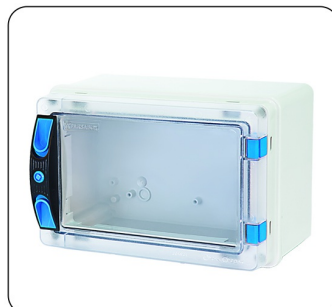
Cabinet with horizontal lid (transparent) Size: 190×280×164 IP66 Code: T18271
