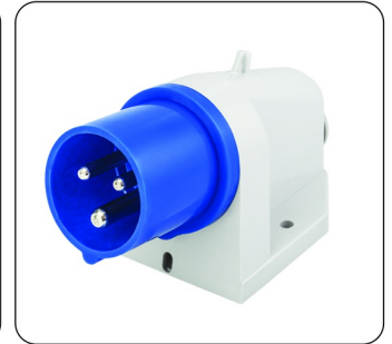
Appliance Inlet 2P+E-16A-6h/250V~ IP44 Code:600
