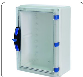
Cabinet with vertical lid (transparent) Size: 600×400×210 IP66 Code:T60401
