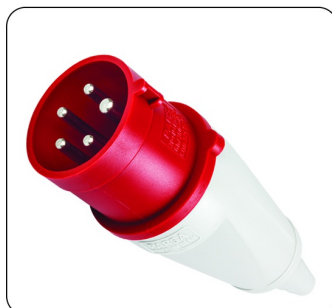
Plug 3P+N+E-32A-6h/415V~ IP44 Code:325
